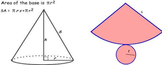
**Example 3:** Determine the surface area of this cone if the diameter of the base is 3cm and the slant height is 9cm.
