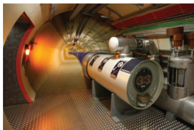
Figure 1 Particle accelerators, such as the Large Hadron Collider, increase particle speeds to nearly the speed of light. The resulting increase in the inertia of the particles means that strong magnetic fields are needed to bend the trajectories of the particles into a circle.
