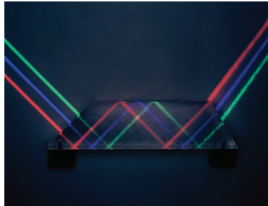
Figure 13 Total internal reflection can be used to make devices that change the direction of a light beam.
