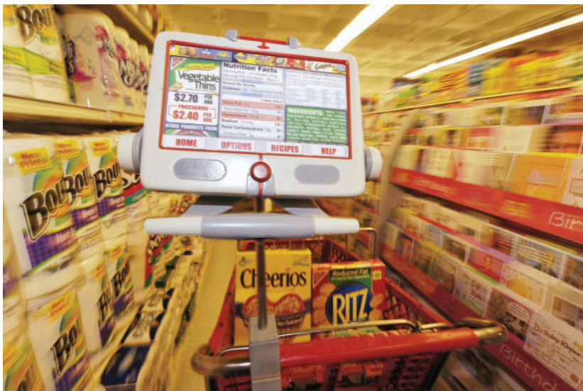
Figure 2 A shopping cart equipped with an RFID scanner and display
