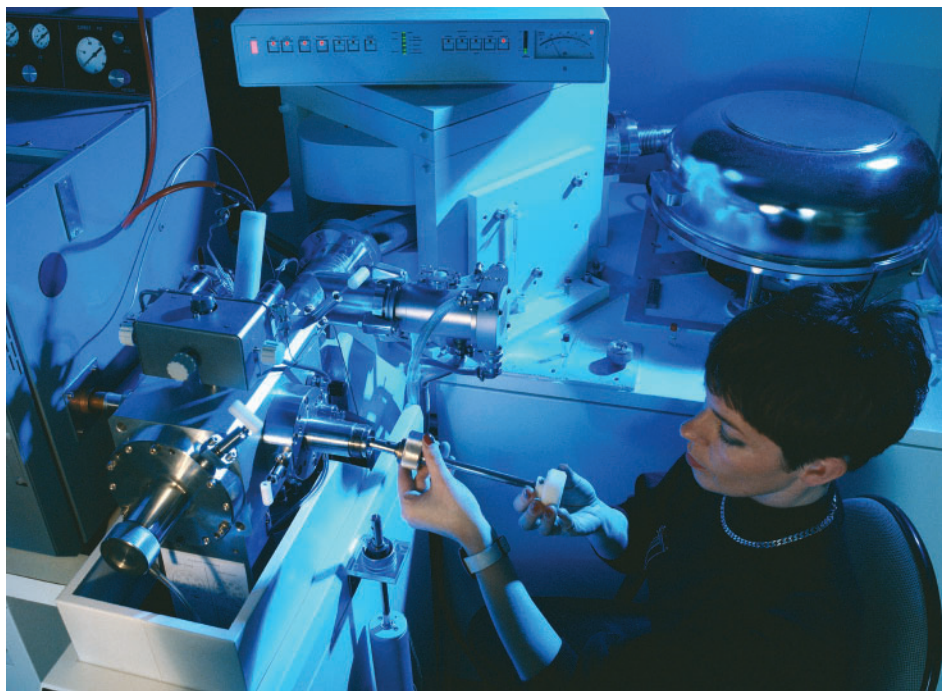
Figure 1 A scientist inserts a sample into a mass spectrometer.
