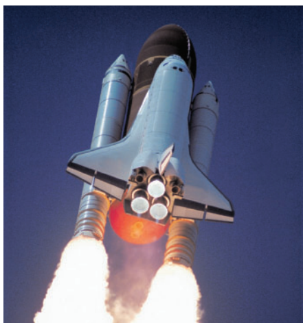
Figure 4 The momentum of combusted gases ejected from the rocket is balanced by the forward momentum of the rocket.
