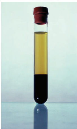
Figure 4 A centrifuge rotates at an extremely high rate, producing a large centripetal acceleration for the contents of the test tubes. As a result, the higher-density cells move to the outer end of the tube and separate.
