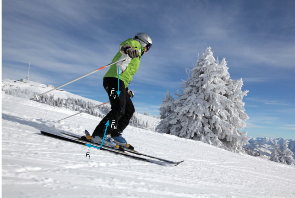
Figure 1 The forces on this skier are gravity, the normal force, and friction. Compared to the other forces acting on the skier, air resistance is negligible here. These forces can be broken into components parallel and perpendicular to the hillside to analyze the motion of the skier.
