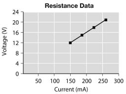
The slope of the line connecting the data points represents the resistance. For example, the line passes through the data points (12 V, 151 mA) and (18 V, 226 mA). First convert the current to amperes to find the resistance in ohms:
