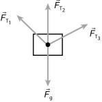
**14. (a)** Answers may vary. Sample answer: Since muscles are made of small fibres, they are not rigid. Like ropes and strings, they can only pull on an object, not push on an object. Therefore, muscles can only cause tension forces.
