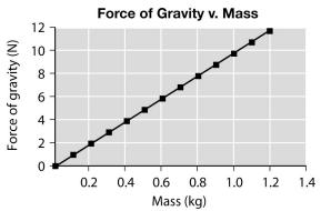
**B.** The slope of the line of best fit is 0.98. The slope represents the rate of change of gravity on objects of different masses. The heavier the objects are, the stronger the force of gravity is.
