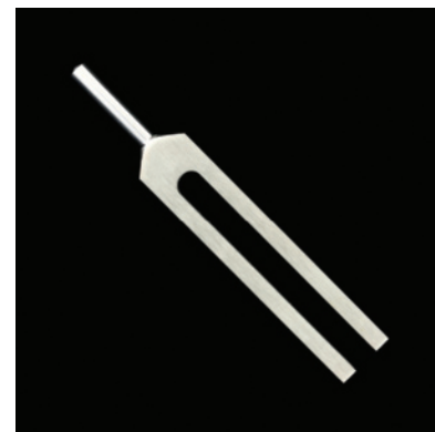
Figure 2 Tuning forks are available in different frequencies. A light tap to one tine (prong) of the fork sets both tines vibrating at a particular frequency.
