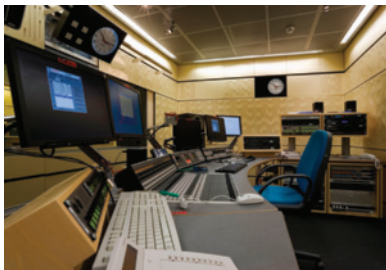
Figure 1 The walls and shapes of recording studios are carefully designed to ensure that the sound going to the microphone is a true representation of the work of the musician. The walls contain materials that absorb sound.
