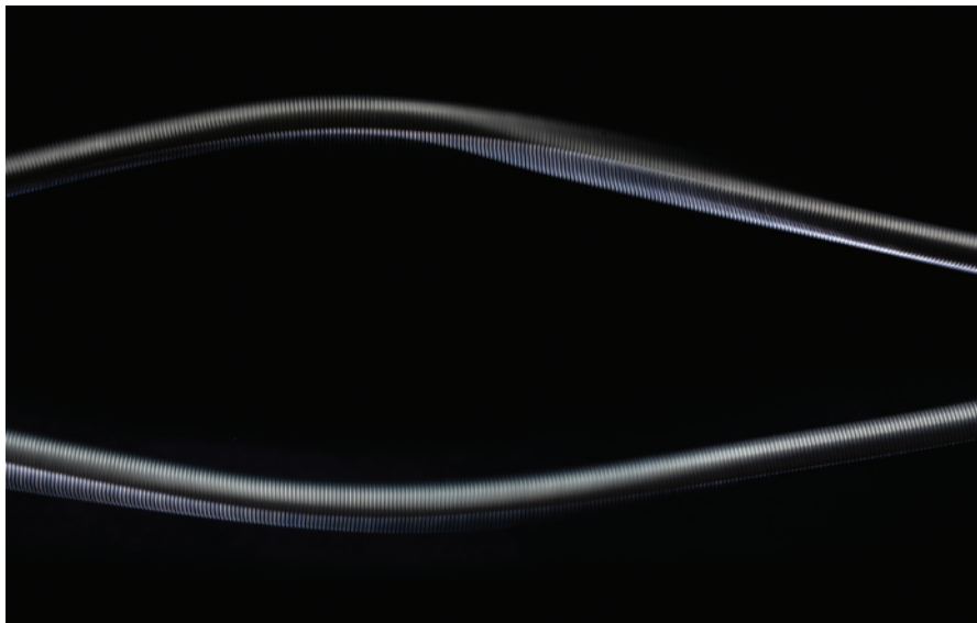
Figure 1 In this image of a single vibrating guitar string, the particles in the string are moving up and down, and the energy is flowing back and forth along the string.
