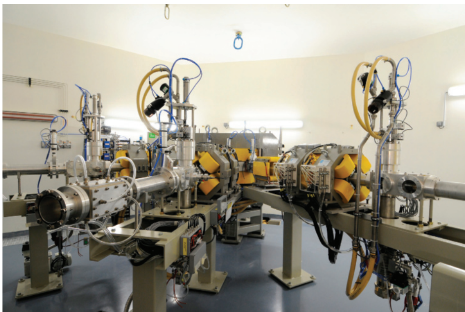
Figure 1 A cyclotron is a device that accelerates particles to very high speeds approaching the speed of light. The high-energy particles that are produced can be used for research experiments, as well as medical treatments.
