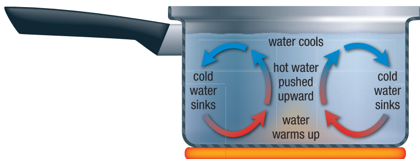
Figure 4 Convection currents cause the liquid in the pot to move around, spreading the thermal energy evenly.
