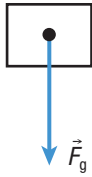
Figure 5 This FBD shows an object in free fall, with no air resistance acting on it. The net force on the object is the force of gravity. The acceleration of the object is equal to the acceleration due to gravity.
