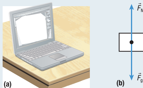
Figure 3 (a) System diagram of a computer on a desk (b) FBD of the computer
