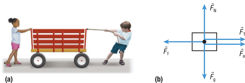
Figure 4 (a) The system diagram of a wagon and the two children pushing and pulling on it (b) The FBD showing all the forces acting on the wagon
