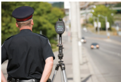
Figure 1 A laser speed device can accurately measure the speed of an oncoming vehicle.
