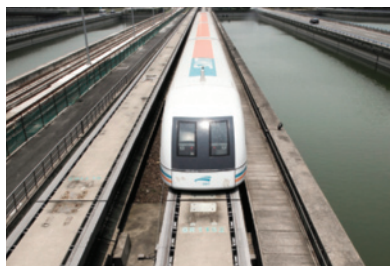
Figure 1 This train uses magnetic levitation to float above the tracks and avoid friction.
