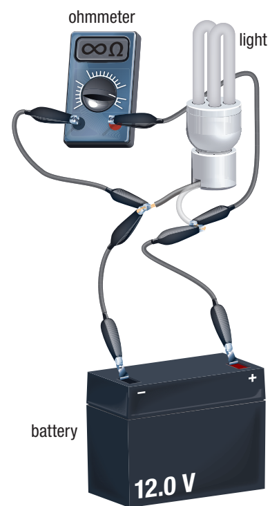
Figure 3 The load in this circuit is not functioning. The display on the ohmmeter shows that the reading is off the scale of the device. Note that the circuit must be switched off before measurements are made with an ohmmeter.
