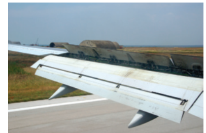
Figure 2 Aerodynamic brakes cause normal vibrations in aircraft.
