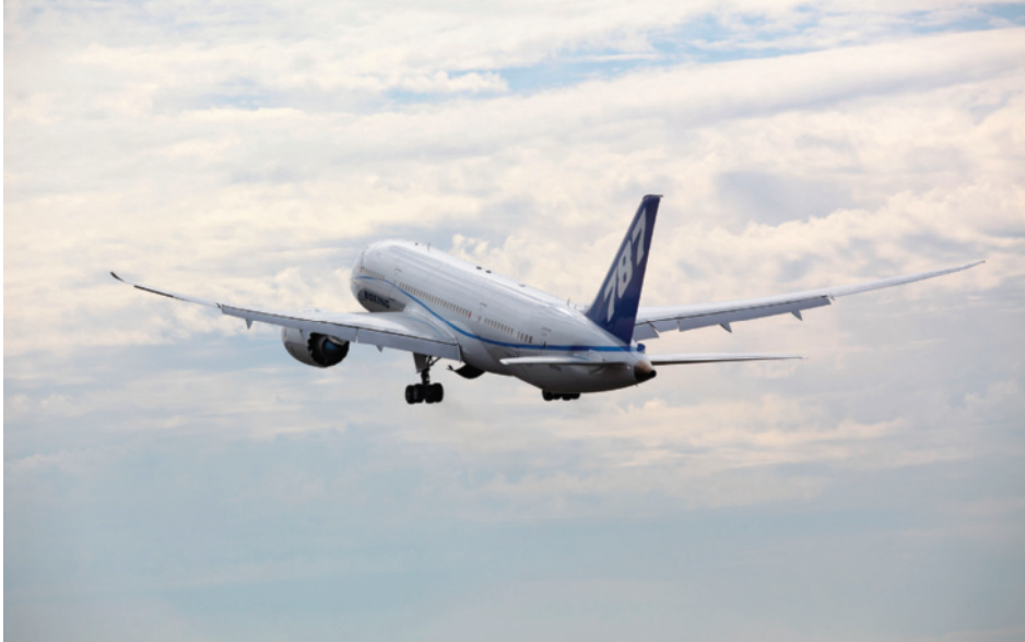
Figure 1 The wings of commercial airliners are designed and constructed to be flexible. Most wave motion that the wings experience is accounted for in the design.
