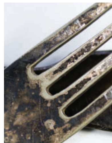
Figure 1 Mixing copper with silver makes the silver harder but also causes it to tarnish.
