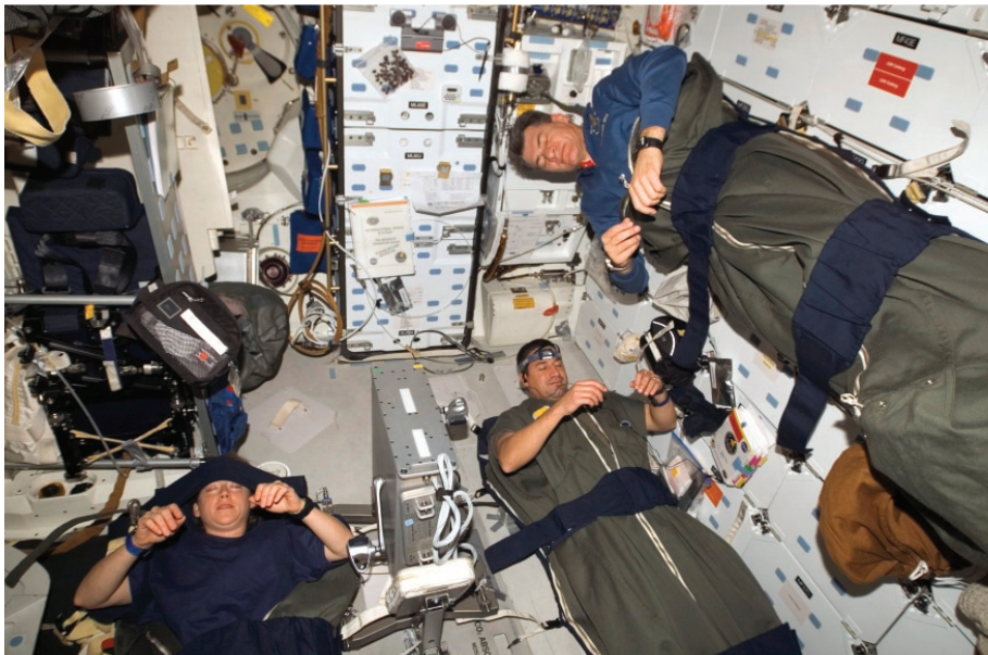
Figure 9 This wall-mounted sleeping bag has arm restraints to keep arms from floating around while astronauts sleep.
