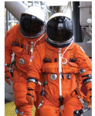
Figure 4 These suits contain a helmet with communication gear and oxygen, as well as a parachute pack, life raft, and life preserver in case of a re-entry emergency.
